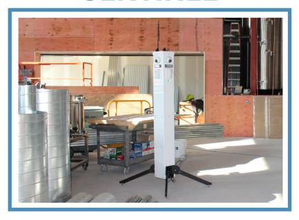
The Sentinel is a self-contained site protection product designed to defend an area. This system captures and retains video at 360°. Using MPS Defense System, the Sentinel is able to arm and disarm one or multiple units on a specific location. Once armed, detection is active using video analytics and infrared motion sensors to detect motion around the unit. When activity is detected, users are notified and provided snapshots.
